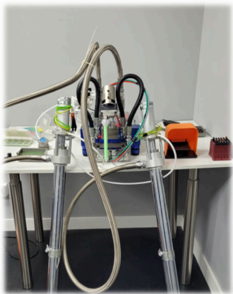
INNOMIX LCP WITH TWO PISTON PUMPS FOR 200 KG DRUM
