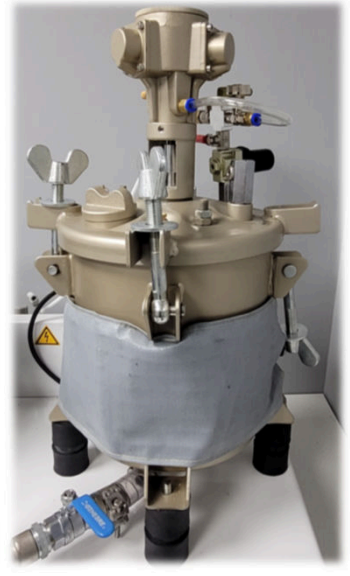
STAINLESS STEEL 10 LITER TANK WITH PNEUMATIC AGITATOR AND HEATING JACKET
